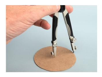
With the point in the middle of the circle, move the pencil end of the compass so that it lines up with the edge of the circle. Mark the circle in this place.
