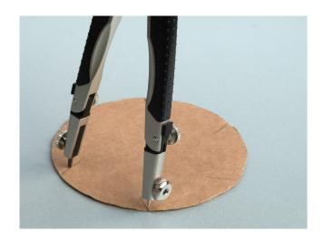
3. Repeat step 2 around the circle until you get back to the first mark you made. You should have 6 marks in total, equally spaced.
