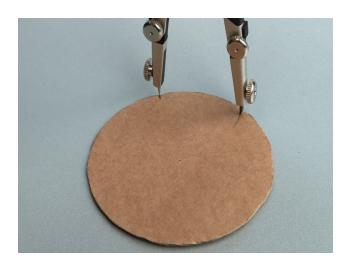
2. Without changing the width of the compass, place the point on the mark you just made. Swing the pencil end of the compass clockwise and make a mark where the pencil naturally meets the edge of the circe.
